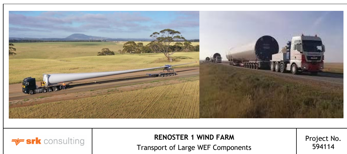
Figure 2-14: Examples of Transport of large WEF components – blades (left) and tower sections (right)
