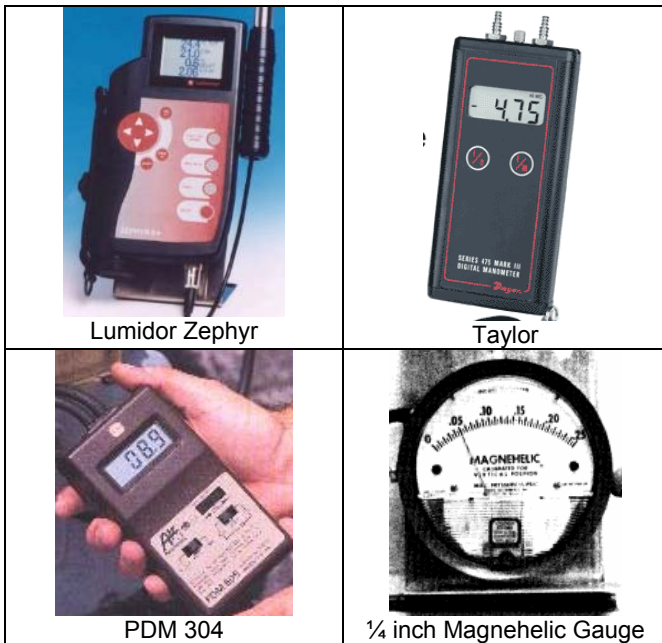
Figure 2: General Types of Manometers
