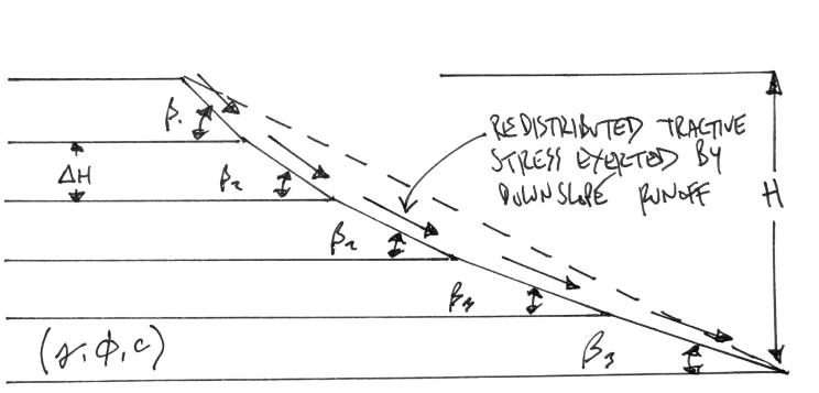
Field and lab studies show that convex-concave ("catena" profile") slope profiles are more (geomorphically) stable and generate less sediment than uniform planar slopes.
