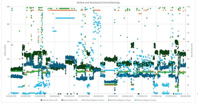
Record of VOD system changes of regulator settings, airflows
