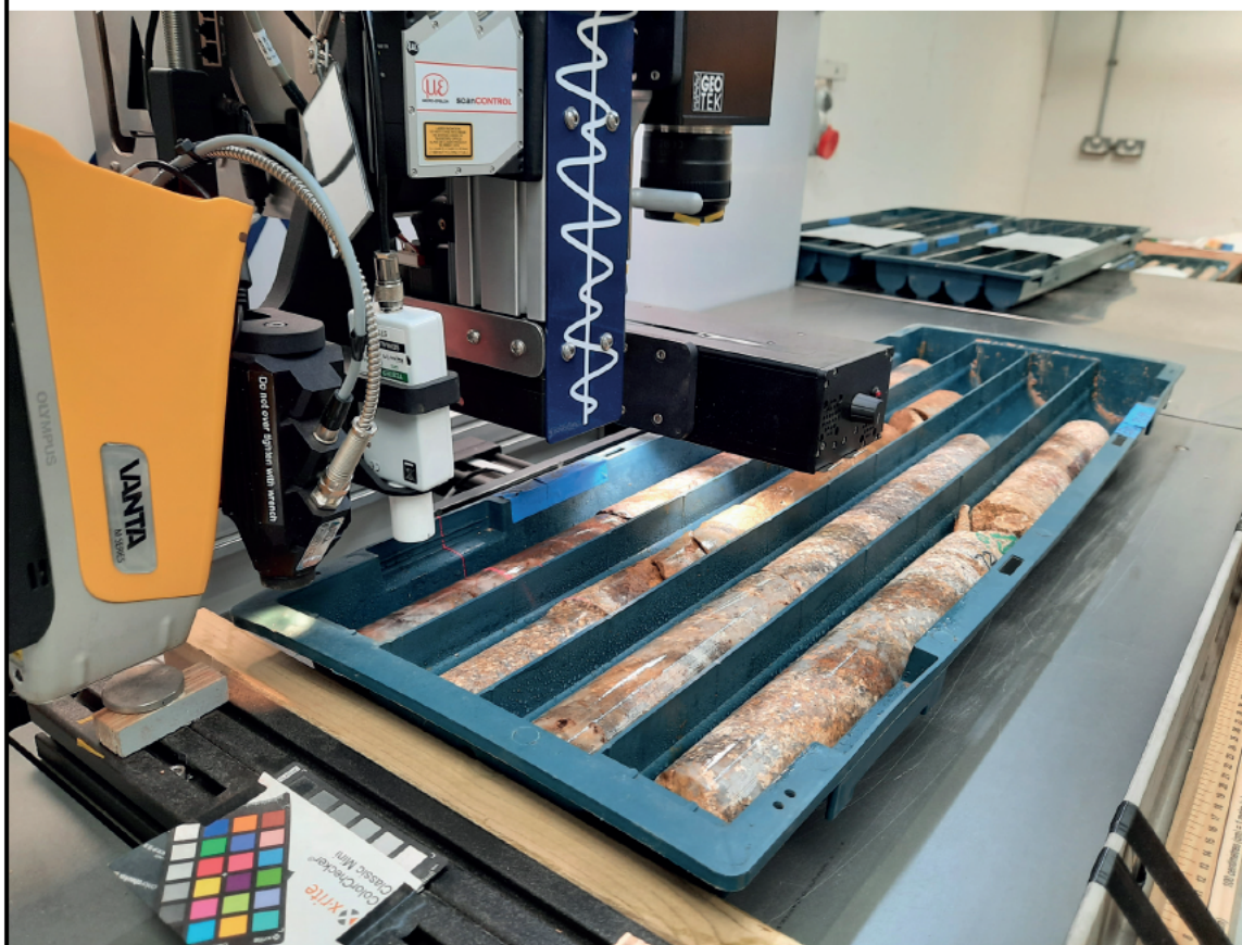
Geotek Boxscan analysing core with an integrated Vanta pXRF
