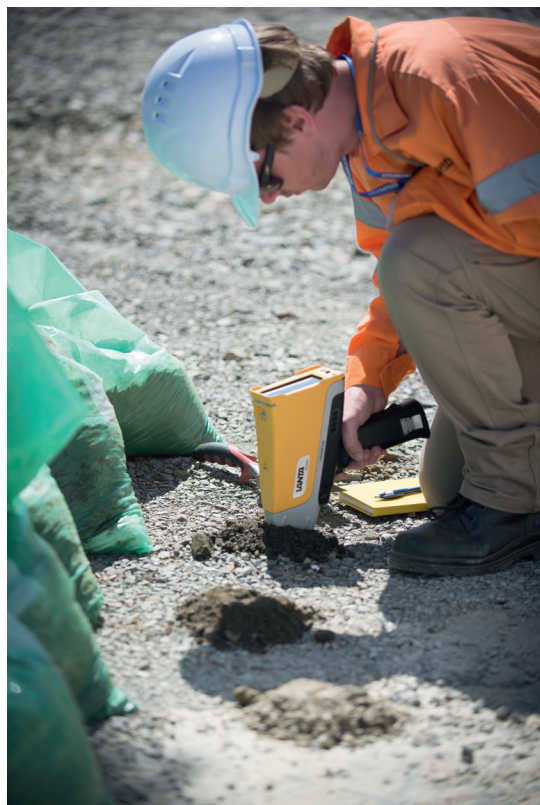
Olympus Vanta pXRF analyzing RC samples in the field
