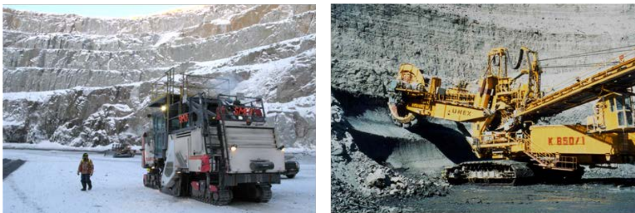
Figure 6 Wirtgen cutter tested by Ekati mine at Fox pit (left) and bucket wheel excavators used for trial mining at Udachnaya mine in Siberia (right), both implemented to reduce diamond breakage
