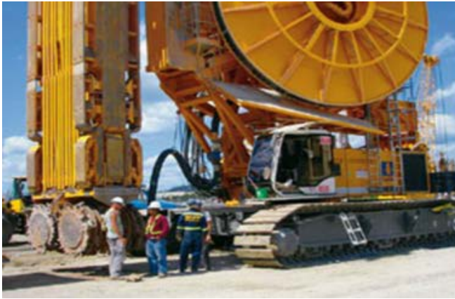
Figure 7 Bauer trench cutter (left) and new continuous miner for undersea mining (right)
