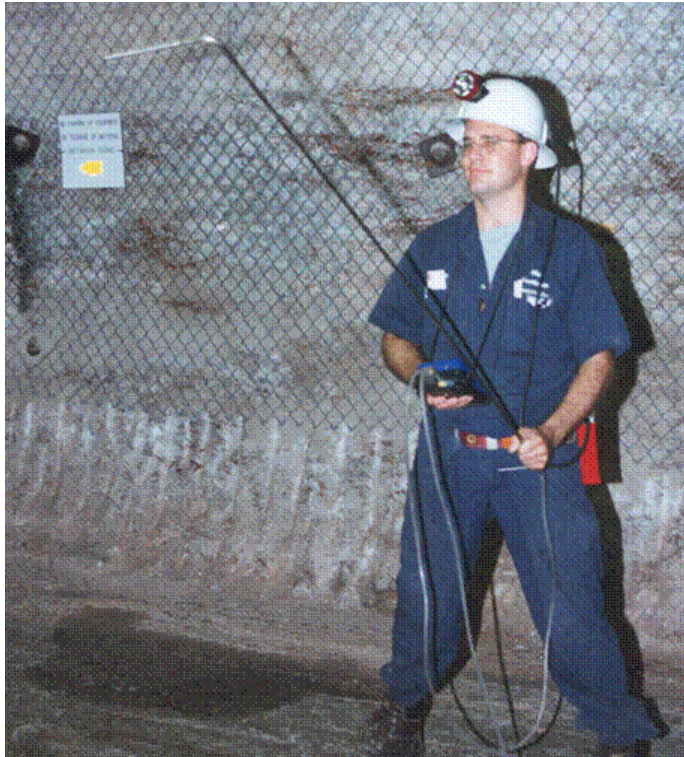
Surveyor with pitot tube and manometer.
