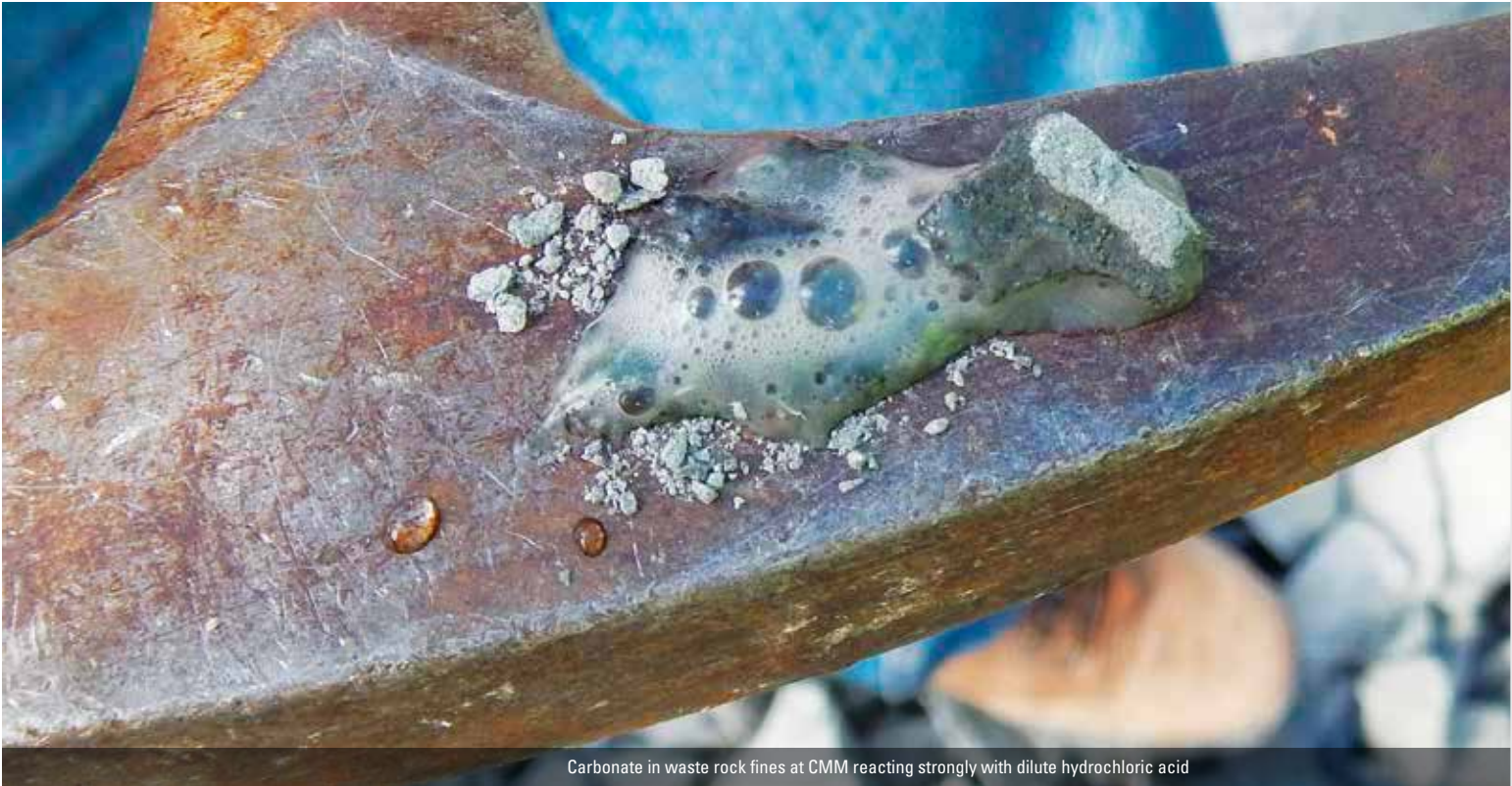
Carbonate in waste rock fines at CMM reacting strongly with dilute hydrochloric acid
