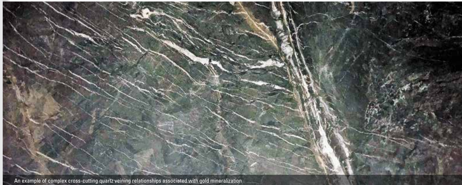
An example of complex cross-cutting quartz veining relationships associated with gold mineralization
