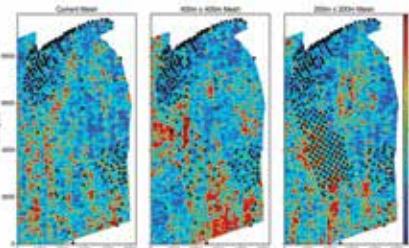
a) Current and Proposed Drilling Meshes Against Possible Seam Thickness Scenarios
